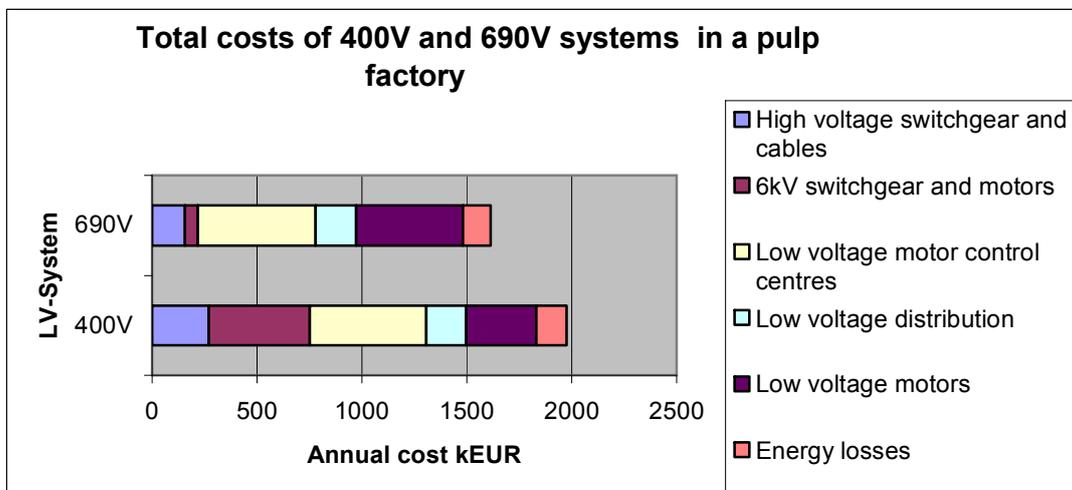
Comparison of total investment and power losses of 400 V and 690 V systems calculated on an annual basis during 15 years running time in a pulp factory
