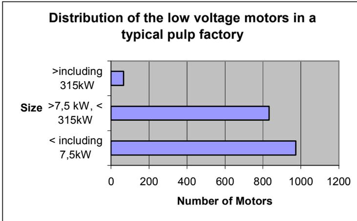
Low voltage motors in a typical pulp factory divided into main categories
