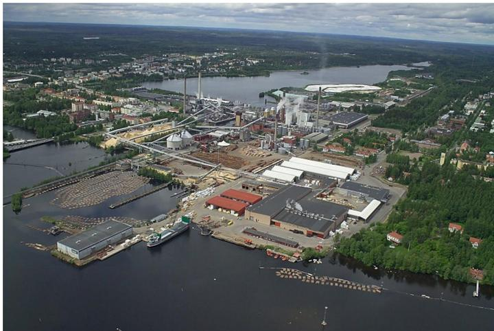
*The power consumption of the Stora Enso paper mills in Varkaus is about 150-160 MW. About 20-25 per cent is produced at the mill and the rest comes from the national grid. The amount of squirrel cage motors is about 7000. The unit that needs most power is the Thermo Mechanical Plant (TMP). The effect of the main grinder motors at stages 1 and 2 of the new line in the TMP is 64 MW in total.*
