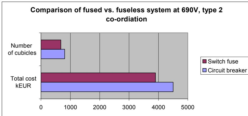
Comparison of total cost and number of cubicles of motor control centers in a green field pulp factory project by 690 V, 50 kA and type 2 co-ordination.
